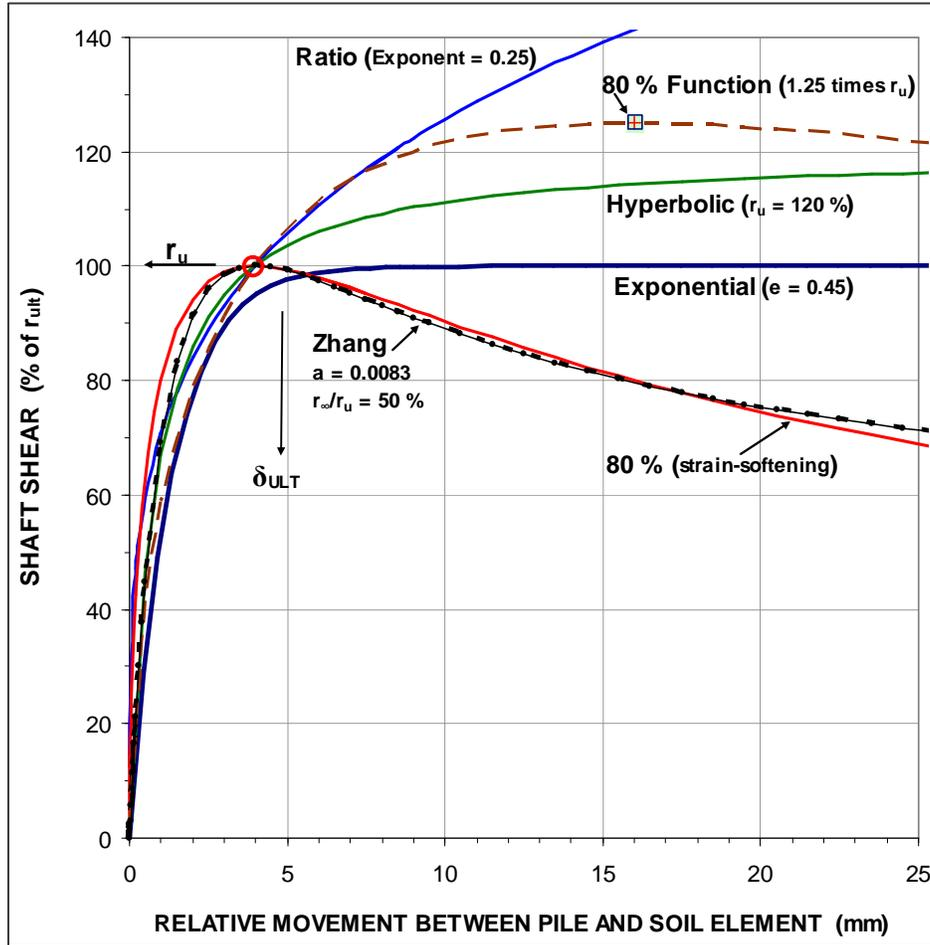
**Suggested t-z and q-z functions for load-movement response<sub>f</sub>**
